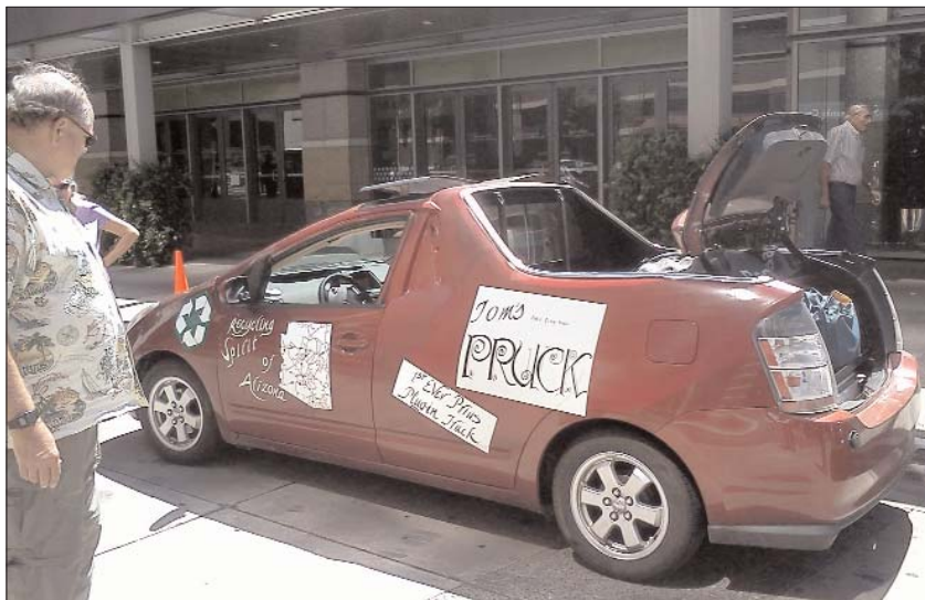
Jerry Asher admires the PRUCK, a 2005 Prius that has been converted into a plug-in hybrid pickup truck.
