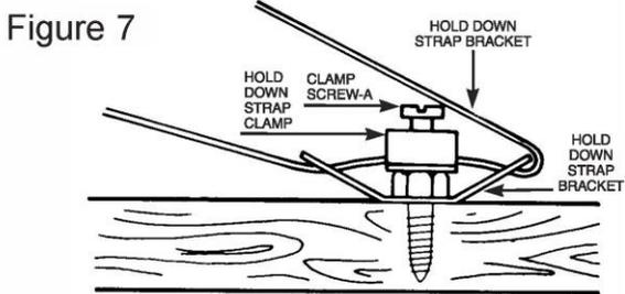
and bend it back toward the clamp. Refer to Figure 7. Slip the loose end of the strap through the strap clamp and pull it tight. Clamp screw (A) should be tightened securely, but not over-tightened to the point where the clamp is distorted. Refer to Figure 8. Bring the remaining strap end across the collector face, passing through
