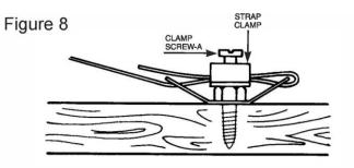
both slots in the bracket located on the other side of the collectors. Pull the straps taut against the face of the collector. Repeat this procedure for the remaining hold-down strap. Refer to Figure 9.
