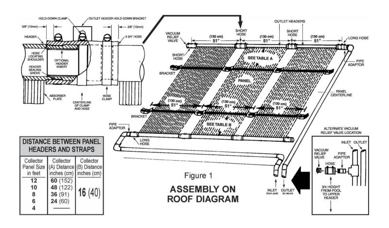
1) Determine the position of the last outlet header hold-down bracket for the row of collectors. Mark this point on the roof. The collector outlet headers will be located approximately 1" (25mm) below this mark. Refer
