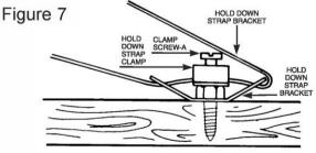
and bend it back toward the clamp. Refer to Figure 7. Slip the loose end of the strap through the strap clamp and pull it tight. Clamp screw (A) should be tightened securely, but not over-tightened to the point where the clamp is distorted. Refer to Figure 8. Bring the remaining strap end across the collector face, passing through
