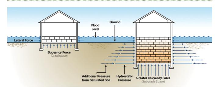
The deeper a basement or crawlspace, the greater the hydrostatic pressure pushing against it. Image: www.yourfloodrisk.com.
