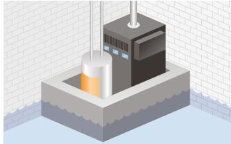
Because of hydrostatic pressure, component floodproofing barriers should designed to a maximum of 3 ft. Image: Colin Hayes.
