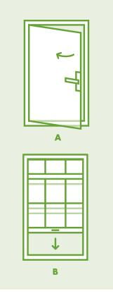
Casement windows (above) open on a hinge and provide a tight seal; doublehung windows open vertically and are usually less airtight. Consider these features:
