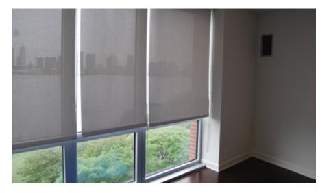
In the winter, the sun is lower in the sky and the direct solar gain is beneficial. At night, window treatments like exterior storm windows, exterior roller shutters, interior glazing panels, interior curtains or insulating blinds can help reduce heat loss.
