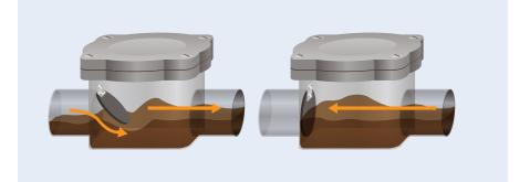
Backwater valves are situated above the external sewer line and should be installed in buildings that have sewer connections below the highest manhole cover in the sewer system, especially if the property is within the Special Flood Hazard Area (SFHA). Although sewer blockage can occur any time, it is most likely to happen during storms when large amounts of water and debris move through the system.
