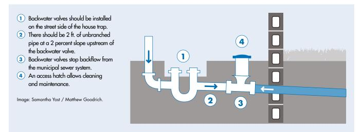
Depending on its size and the configuration of drain piping in the basement, a building may have just one backwater valve connected to the main sewer line, or separate valves may be installed on different lines and drains. Backwater valves should be enclosed in a masonry pit with a waterproof cover giving access for cleaning and maintenance.
