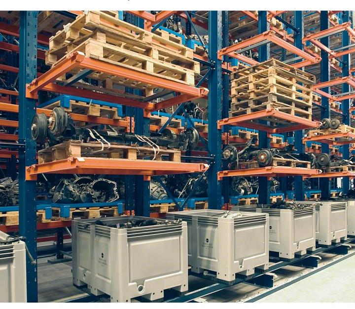
Robust design, high stability. The uprights and feet are made from hot rolled IPE profile and are bolted together to form a rigid cantilever frame. Large footplates ensure even distribution of the load to the floor.
