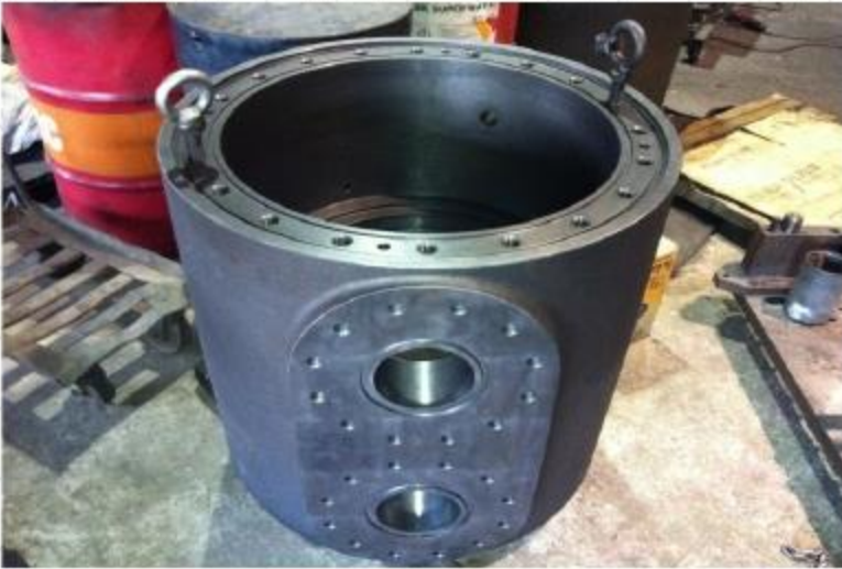
BUSHING HOUSING: A536 Gr.60-40-18
