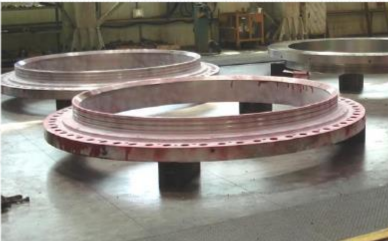
DOWNSTREAM FLANGE: A182 Gr.F304(Forged)
