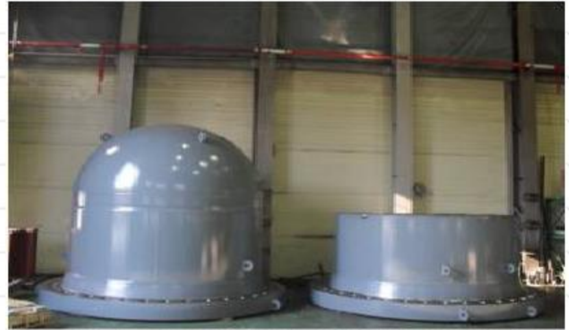
UPSTREAM EXTENSION with PRESSURE HEAD: A516 Gr.70 & A537 Cl.2(Fabricated)
