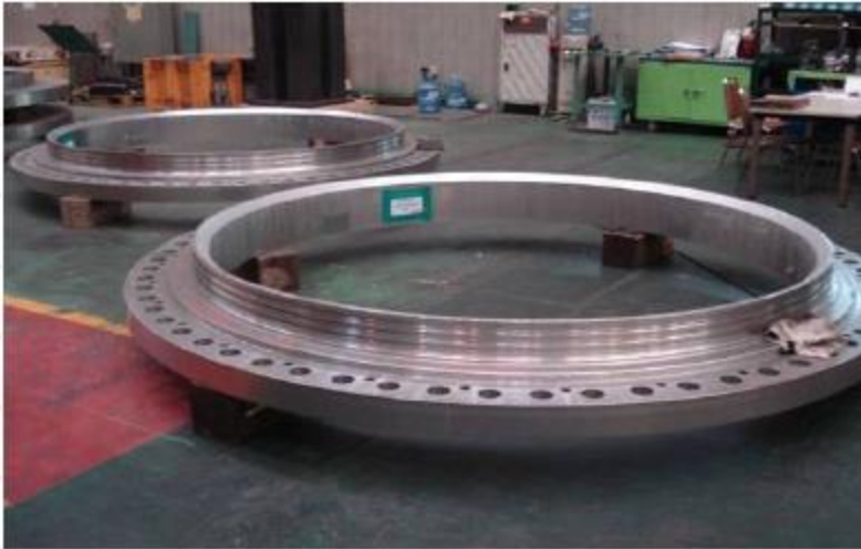
UPSTREAM FLANGE: A182 Gr.F304(Forged)
