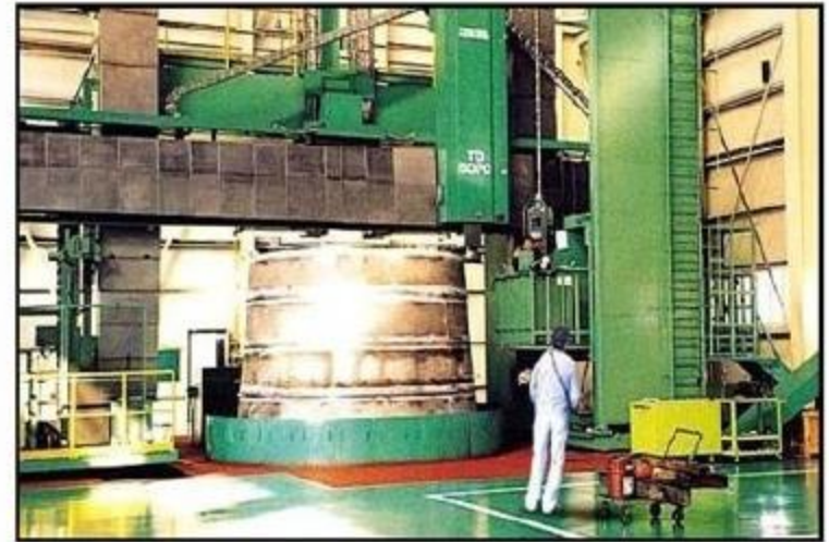
Gas Turbine Diffuser
