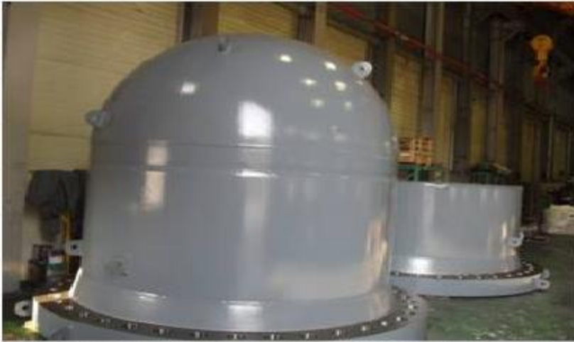
UPSTREAM EXTENSION with PRESSURE HEAD: A516 Gr.70 & A537 Cl.2(Fabricated)
