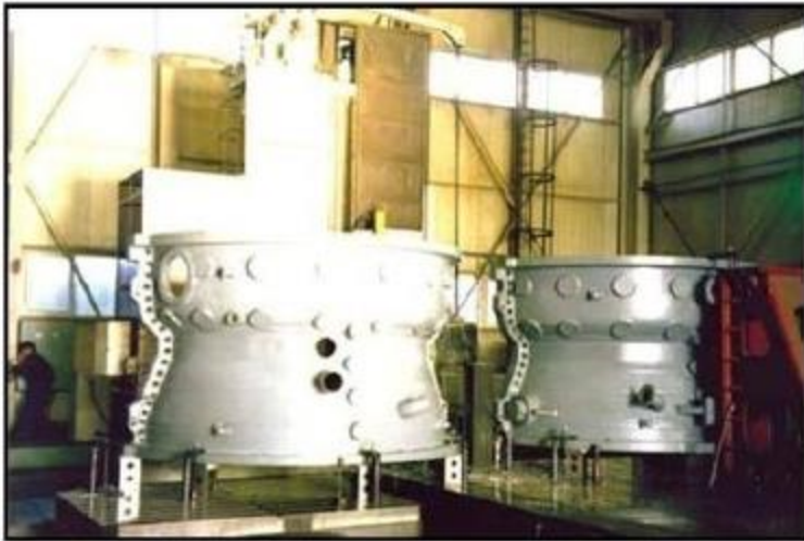
Gas Turbine Casing
