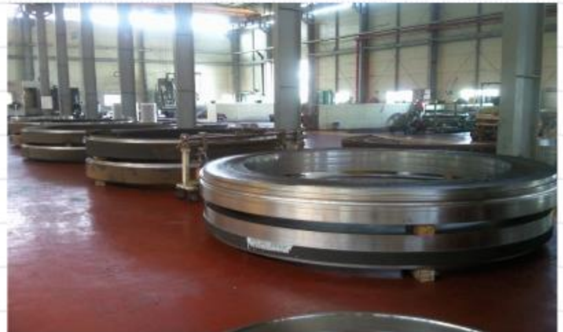
UP/DOWNSTREAM FLANGE: A182 Gr.F304(Forged)
