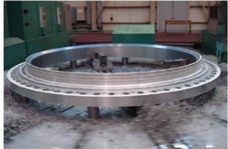
UPSTREAM FLANGE: A182 Gr.F304(Forged)
