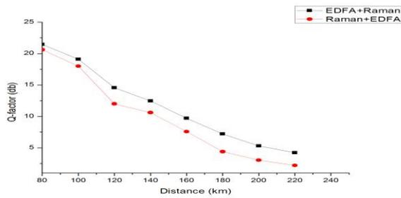
Fig.5:Q-factor v/s distance graph with EDFA+RAMAN and RAMAN+EDFA amplifies.
