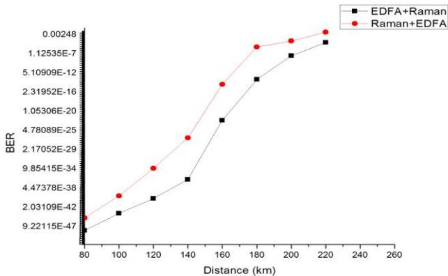
Fig.6: BER v/s distance graph with EDFA+RAMAN and RAMAN+EDFA amplifies.
