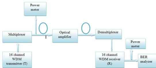
Fig.2: Block diagram of simulation setup
