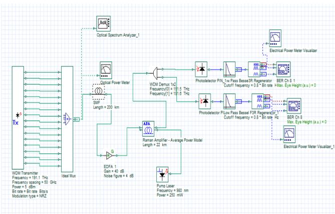
Fig.3: Simulation setup using EDFA+RAMAN amplifier
