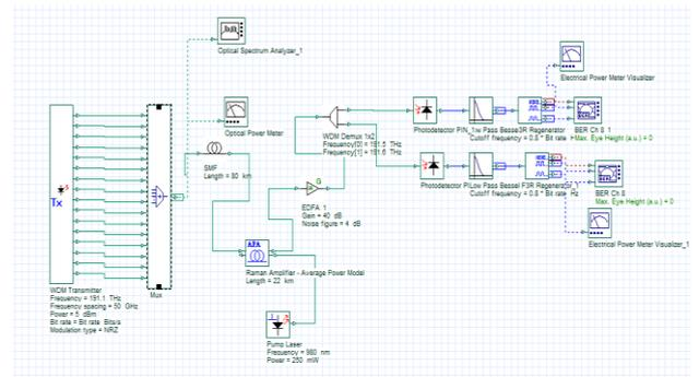
Fig.4:Simulation setup using RAMAN+EDFA amplifier
