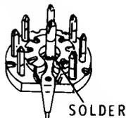
( ) Install a 9-pin tube socket with ground clip at V1.
