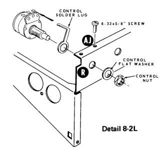
control nut. Form the control solder lug against terminal 1 of the control. Before soldering, check to see that the formed lugs will fit under the chassis lip at R. Solder lug 1 (S-1), and then remove the control flat washer and control nut.
