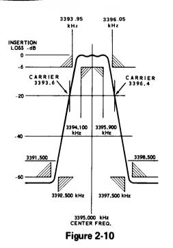
intelligence. The carrier amplitude itself is further reduced 20 dB by the crystal filter. This attenuation plus the ettenuation of the belenced modulator gives an ultimate carrier attenuation of at least 50 dB. (The apparent frequency discrepancy here in sidebands and carrier is overcome later, when the sidebands ere inverted in the second mixer.)
