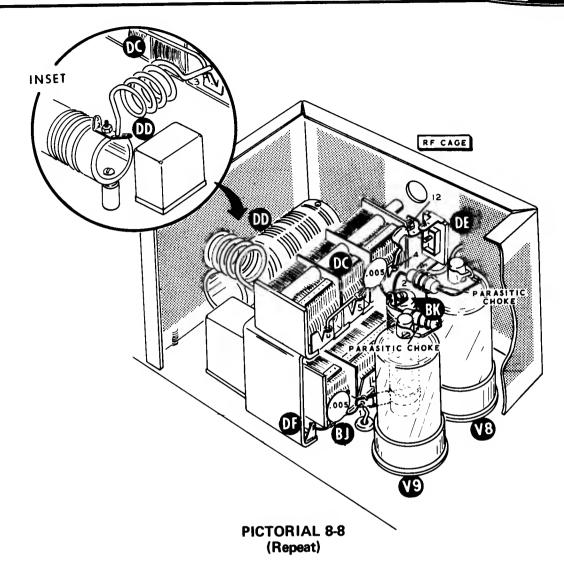
() Refer to Detail 8-8B and cut 5/8" from the long end and 1/4" from the short end of the 10 meter final tank coil (#40-549).
