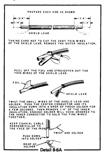
() At the other end of this cable, connect the center conductor to F (S-1) and the shield lead to the ground foil at GK (S-1) on the modulator circuit board.
