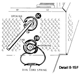
() Position pulleys DC and DB with their openings as shown in Detail 8-15F.
