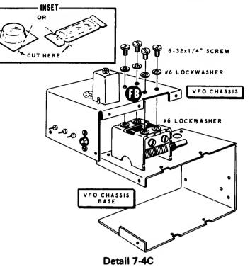
Refer to Detail 7-4C and mount the variable capacitor at FB on the VFO chassis as directed in the following steps.
