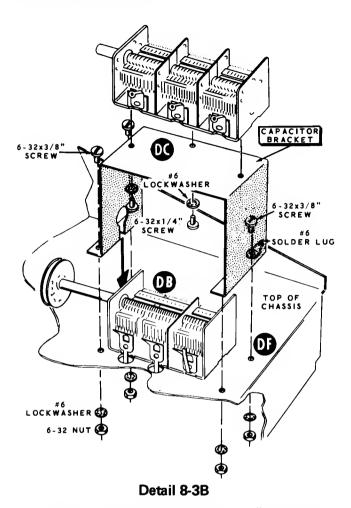
Install the pulley with the small hole (#100-19) flush with the end of the shaft of capacitor DB. Use an 8-32 x 1/4" setscrew. Fully mesh the plates of the capacitor and position the opening in the pulley as shown.
