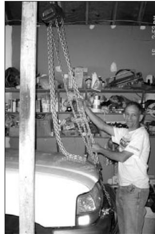
*Using hydraulic jacks Vince dropped the battery pack onto a low slung creeper with castors and then hoisted the front of the truck up using the pictured bumper attachment. The truck raised from the front providing clearance to roll the pack out to the side.*
