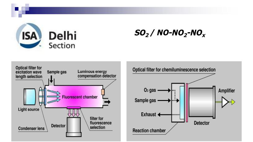
UV Fluorescence Detector for SO<sub>2</sub> Chemiluminescence Detector for NO-NO<sub>2</sub>-NO<sub>x</sub>
