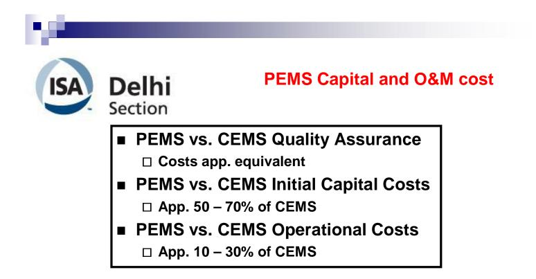
PEMS is in accordance with US-EPA and European Regulations and is already successfully used. PEMS seems to offer an interesting alternative to conventional emission monitoring.
