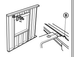
3. Adjust projection of bracket clip by loosening the screw nut (C). Adjust bracket projection as needed. Retighten the screw nut to hold the clip in desired position.
