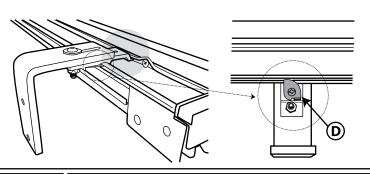
6. Test the cord to assure that rod draws smoothly. Install the floor tension pulley for the cord.
