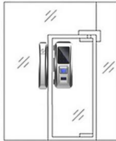
2. For one swing door (other side is glass)
