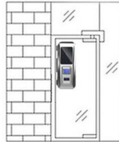
3. For one swing door (other side is wall)
