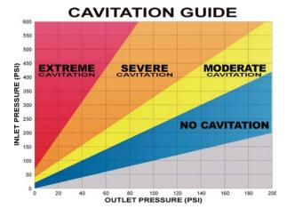
Using the cavitation guide, we can determine the degree of cavitation present in an application and decide if the best solution is a standard valve (when cavitation is not a concern), a single valve with anti-cavitation protection, or a multi-valve approach that takes the pressure drop in two or more stages.
