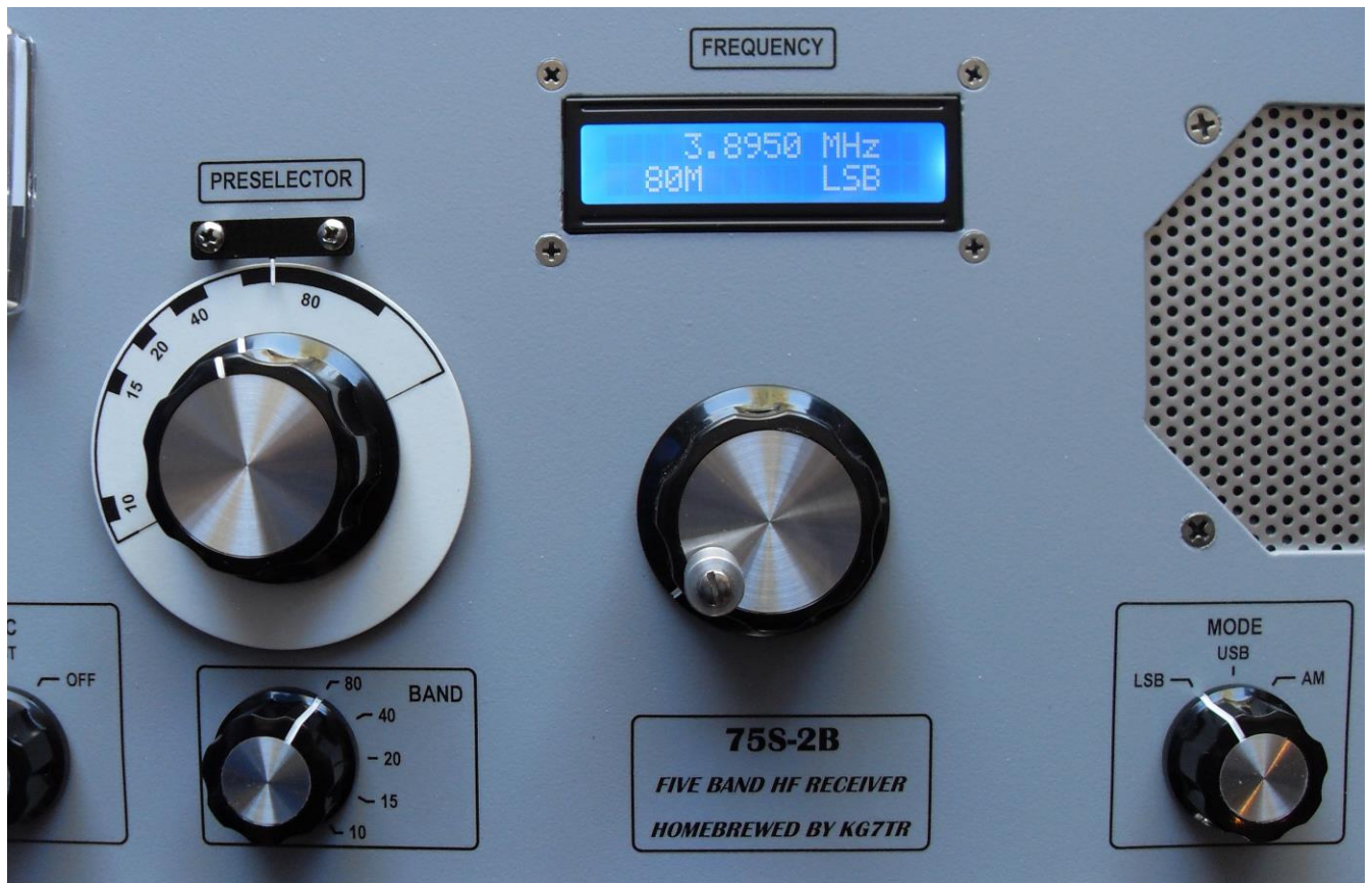
Figure 5: Close Up of Preselector and Main Tuning Controls
