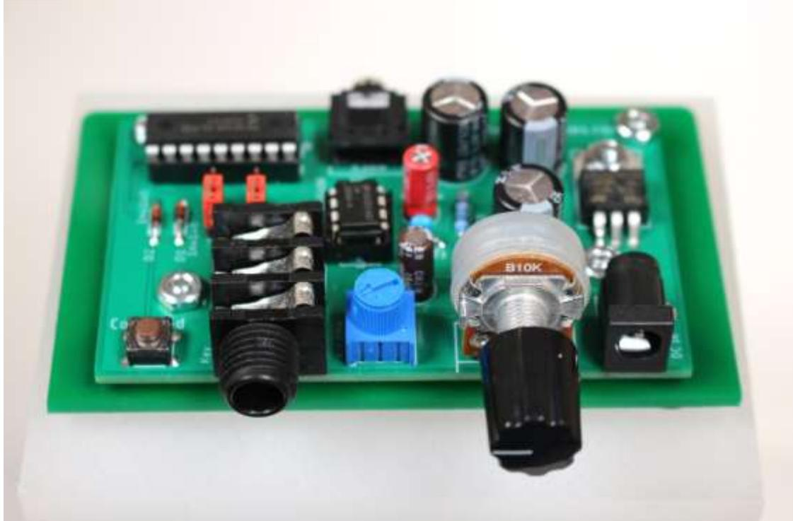
The CMD push switch (located on the left edge of the PCB at the front, is used to access the more advanced features of this oscillator; this switch is pressed once to activate 'Command Mode' as explained below.
