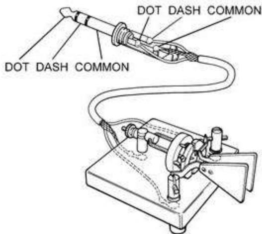
Typically dot is connected to the Tip and Dash to Ring with the common to the sleeve.
