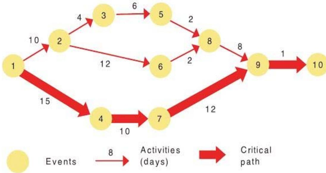
**Figure 2: Current Sample CPM/PERT Network Diagram**
