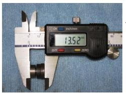
This closing shim measures 3.52mm (13.52mm minus the 10.00mm of the closing shim-measuring tool).
