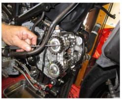
Use a punch and **gently** tap on the Variator to loosen the cam/cam retainers so the camshafts can be removed.
