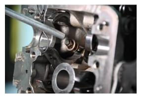
Use the magnet in the kit to remove the half-rings from the valve stem.
