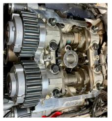
When removing the cam hold-down clamps loosen the inner retaining bolts and then the outer ones. These nuts are  $\frac{1}{2}$  the normal height and it is best to use a 6pt socket.
