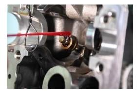
Install the second half-ring onto the valve stem.
