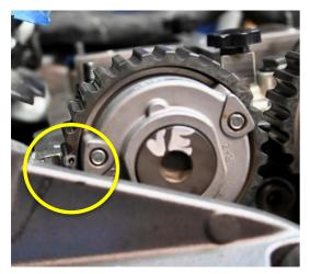
Check the Variator alignment. The marks (dimples) on the Variatiors will align with the plane of the "head flat surface".
