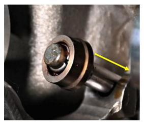
Push the closing shim so it slides (down) on the valve stem, revealing the retaining rings (half-rings).
