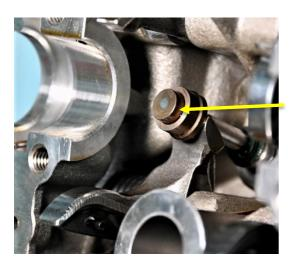
Lift/hold the opening rocker out of the way.
