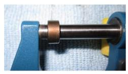
Close the micrometer. Do not over tighten. Press the "zero" button to set the reading to 0.00. Open the micrometer and place the shim on the stationary shaft of the micrometer, with the flat side towards the fixed portion of the micrometer. Measure the opening shim and record the measurement in column [D] of the worksheet. Determine the size of the replacement shim by adding/subtracting column [C] to
