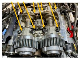
Use gasket sealant on the mating corners where the cam retainers meet the flat surface of the cylinder head for sealing. Torque in two stages to 7ft lbs.
