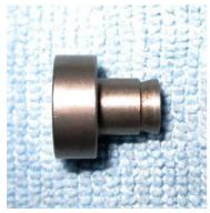
Place the closing shim-measuring tool inside the closing shim and measure. The closing shim-measuring tool fits inside the closing shim and allows accurate measurement with the enclosed electronic calipers. The closing shim-measuring tool adds 10.00 mm to the shim measurement.
