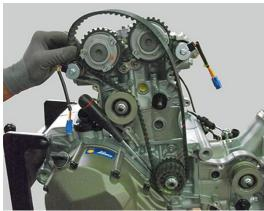
Install the belt on the vertical cylinder: bottom pulley first and work your way up. Use a screwdriver (as shown) to secure it onto the Intermediate Shaft pulley.
