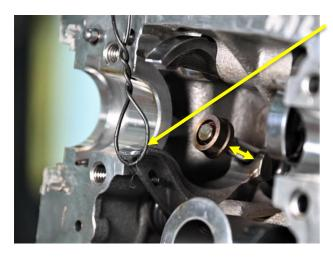
Use safety wire, zip tie, or a screwdriver to lever the closing rocker arm away from the closing shim; relieving pressure on the closing shim. In the photo the closing rocker arm is well away from the closing shim. Remove the opening shim and set it aside.
