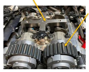
Note: there is spring pressure on the intake cam. Manually rotate the Variator so the flat portion on the camshaft fits neatly into the reaction tool. Use the M6 x 25mm bolts (with plastic knob) to secure the reaction tool to the cylinder head: holding the camshafts in place.
