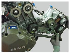
Install the belt for the horizontal cylinder. Place a screwdriver, as shown, to hold the belt in position. If previously removed, fit the belt tensioner , new wave washer and fasten with a new Fuji nut . Do not tighten to torque.
