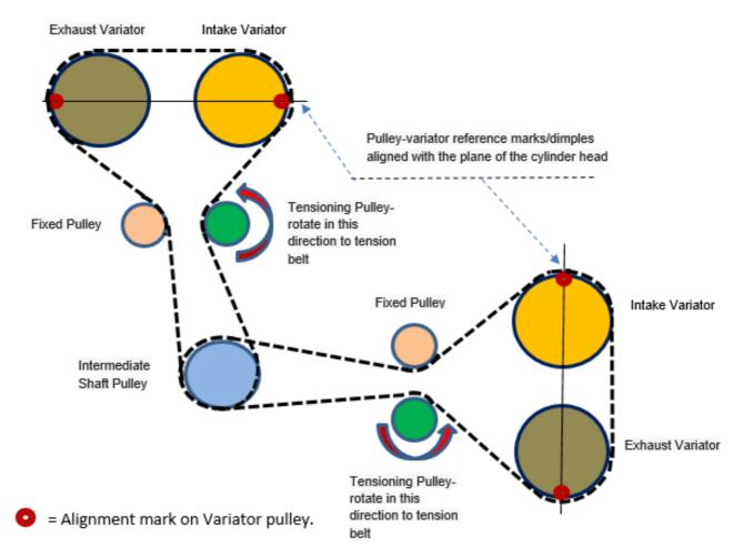
The diagram shows the alignment of the camshafts when properly installed. The crankshaft is locked into position with the crank locking tool (disregard the dimple on the Intermediate Shaft Pulley).
