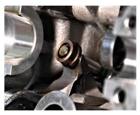
Slide the closing shim up over the half-rings and insure the half-rings remain seated onto the valve stem.
