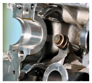
If a closing shim requires replacement, the opening shim will have to be removed from the valve. Remove the opening shim and set it aside, marking the shim's location for reassembly.
