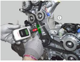
Rotate the crankshaft by 270° counter clockwise to bring the vertical cylinder to TDC.
