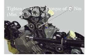
Valve clearance adjustment and belt replacement
