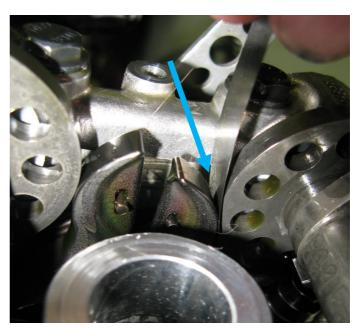
Use the accompanying worksheet (or other preferred method) to record measurements. The worksheet arrangement enables an easy determination about the current valve/shim clearance. It also facilitates determining the new shim size to bring the clearance into specification.
