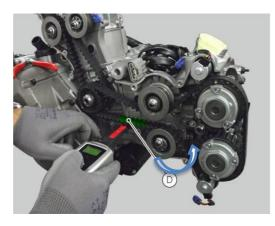
Check the horizontal cylinder belt tension at the indicated point (D). Tension the belt according to the table below.
