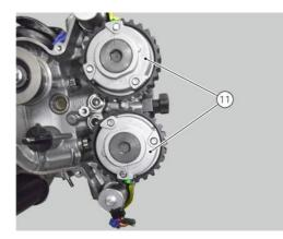
Check the alignment of the Variators (11): the marks (dimples) are aligned with the "head flat surface".
