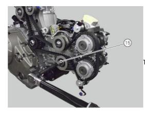
Tighten nut (15) to a torque of 25 Nm (Min. 22 – Max. 28).
