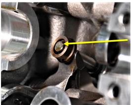
Remove the opening shim by lifting it off of the valve stem.
