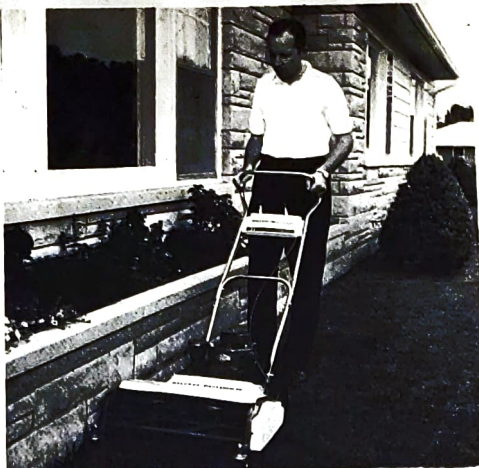
A "trimmer reel" lets you cut close to walls, trees, shrubs and other obstructions, reducing the need for hand trimming. (Moto-Mower)
