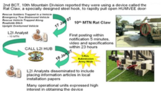
10th Mountain unit of the US Army developed a much needed way to quickly remove the door of a Humvee that had been overturned by an IED, often leaving soldiers trapped inside. This specialized crowbar, which they called the Rat Claw, was attached
