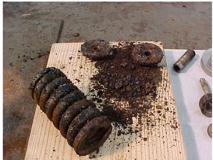
CORRODED SPRING & WASHERS
