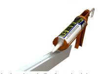
Pre-drill side channels and sill rail, spacing holes a maximum of 18" apart. Apply a 1/8" bead of caulk to the mounting-side of side channels and sill rail at this time. (Caulking is optional.)
