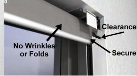
Press and release UP button on remote.\* Ensure that the hard stops are secure, that the shade does not touch the side channels, and that the fabric has rolled neatly onto tube.
