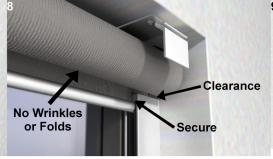
Press and release UP button on remote.\* Ensure that the hard stops are secure, that the shade does not touch the side channels, and that fabric has rolled neatly onto tube.
