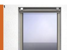
Install roller shade assembly and fascia per their included instructions. Ensure proper fit and function. Remove fascia from its mounting brackets. Leave the roller shade in place.
