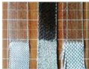
The high crystallinity of the BioMid fiber makes it more transparent than other natural fibers and, therefore, a more likely candidate as a drop-in replacement for glass.
