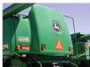
Ashland Performance Materials' (Dublin, Ohio) first commercial grade of its partly bio-based Envirez epoxy resin was used for SMC molding of panels for John Deere tractors and combines. Source: Ashland Performance Materials
