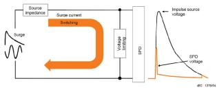
Circuit for voltage-switching devices
