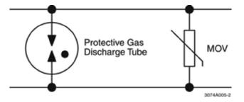
SPDs are classified as T1 or T2 devices correlated to LPZ 1 or LPZ 2 ratings as shown in IEC 62305. They are positioned at the interface boundary of two LPZs. A T1-rated SPD would be inserted on lines entering an LPZ 1 zone from an LPZ 0 zone. Similarly, a T2 device
