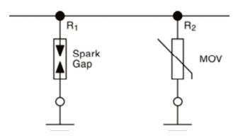
The use of gas discharge tubes in combination with MOVs (Figure ). This combination of components is associated with lightning test current peak values in the range of 50 kA and voltage protection values of approximately 800 V. Compared to the open-air spark gap, the gas discharge tube is environmentally sealed, has a tightly controlled trigger voltage level, faster response time and a lower discharge surge current rating.
