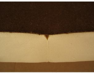
Knit line and V-groove close-up (after conditioning)
