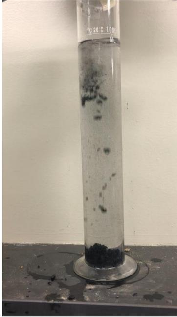
**Figure 16.** *Water Column Condition after adding approximately 30 grams of 0.5% SED-3, 5%PAC-amended sand*
