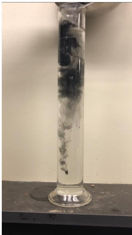
*Figure 9. Initiation of the addition of 5%PAC-amended Sand to Water Column*
