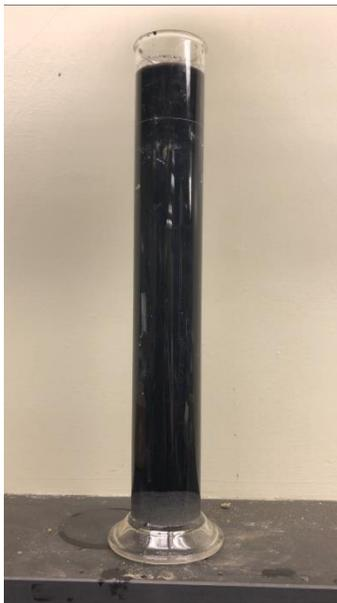
***Figure 11. Water Column Condition after adding 100 grams of 5%PAC-amended Sand***
