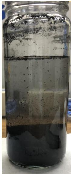
**Figure 14.** 0.5% SED-3, 5% PAC-amended sand sample in water after 60 minutes
