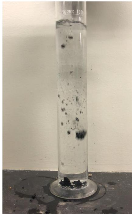
**Figure 15.** Initiation of the addition of 0.5% SED-3, 5%PAC-amended Sand to Water Column
