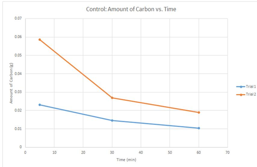
*Figure 7. Control samples Suspended PAC content vs. time*
