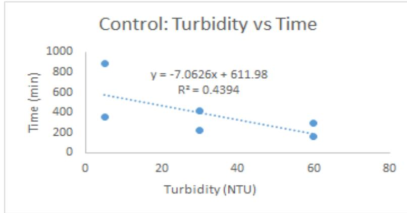
*Figure 6. Control samples turbidity vs. time in duplicate trials*
