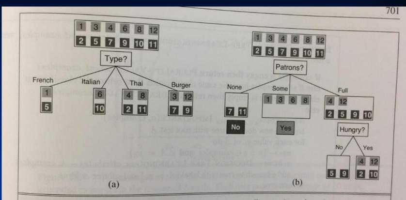
**Figure 18.4** Splitting the examples by testing on attributes. At each node we show the positive (light boxes) and negative (dark boxes) examples remaining. (a) Splitting on *Type* brings us no nearer to distinguishing between positive and negative examples. (b) Splitting on *Patrons* does a good job of separating positive and negative examples. After splitting on *Patrons*, *Hungry* is a fairly good second test.
