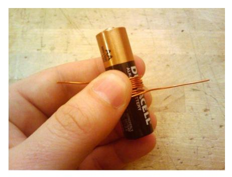
Step1: Wrap the wire around battery, leaving about 2" extra on each end.
