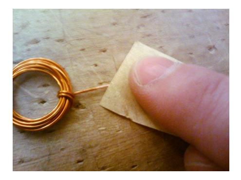
Step3: Using the sandpaper, rub off all of the enamel insulation from one end of the wire.
