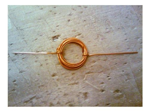
Step4: On the other end, strip off the insulation from one side of the wire, radially. The purpose of this step is to allow the coil to turn on for part of its rotation, and then to turn off on the other part.
