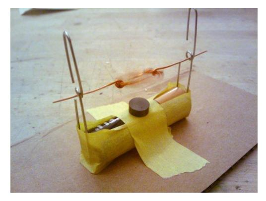
Step8: Now, place the coil on the motor base, sticking one end through each of the loops in the paperclip stands.
