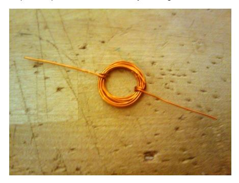
Step2: To keep the coil from unraveling, wrap each end around the coil a few times. The two ends should be on opposite sides of the coil from each other.
