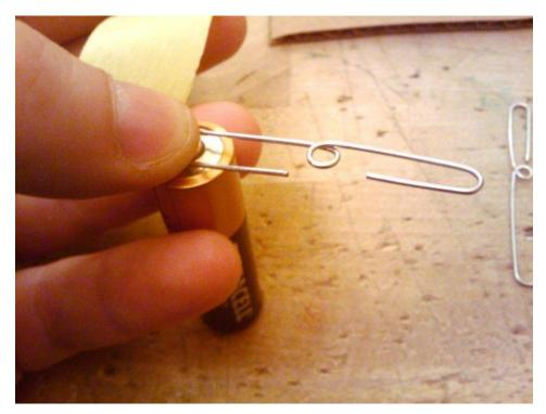
Step6: Next, take one of the paperclip stands, and tape the larger end to the positive battery terminal, making sure that the metal from the paperclip touches the metal battery connector. Then, take the other stand and tape it to the negative battery terminal.
