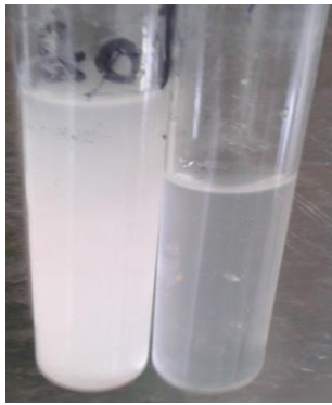
Fig 2: Untreated Dairy wastewater with COD 840mg/l and treated Dairy wastewater with 140mg/l COD value
