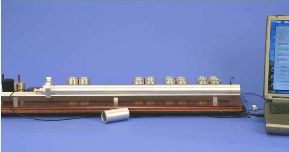
The same computer-based frequency-scanning system will display a whole series of resonant modes, evenly spaced in frequency.
