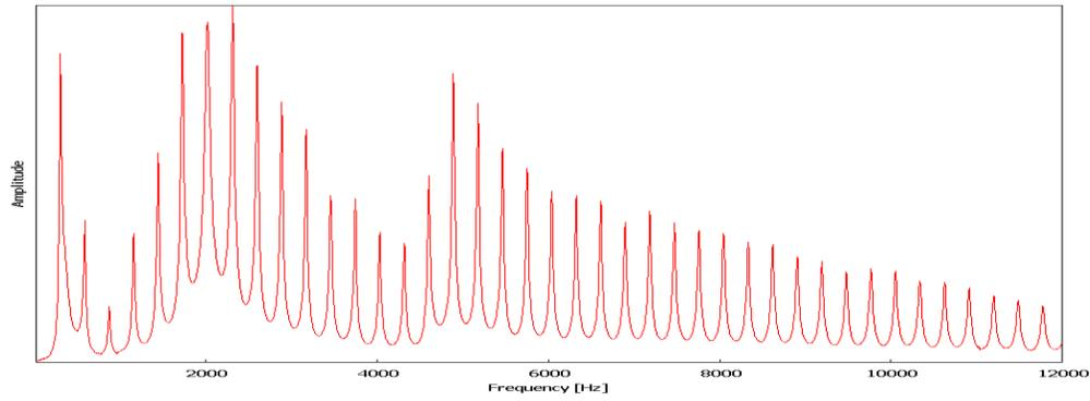
Spectrum measured in a tube made from 12 pieces each 50 mm long without irises.
