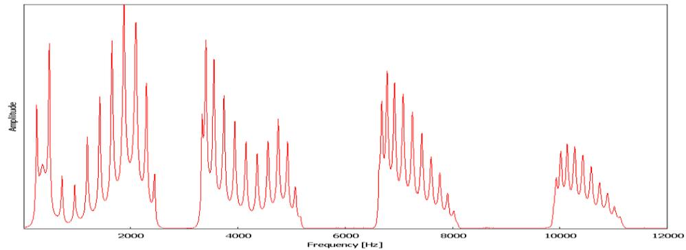
Spectrum measured in a tube made from 12 pieces each 50 mm long and 11 irises which have a diameter of 16 mm.
