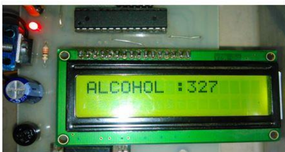
Fig. 5 Normal value of alcohol sensor
