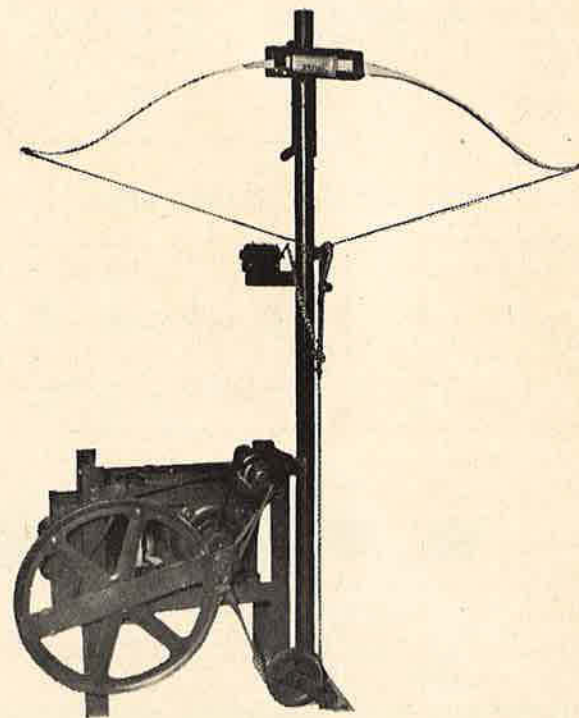
Official pulling machine that drew the Herter Model 21 Farbenglas bow over 250,000 times. At the end of the test, bow showed no signs of weakening, undue stress, crushing, splitting or fibre breakdown, establishing a record.
