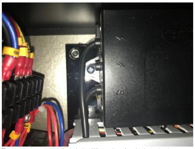
There are two ways to install new ignitor. What we have found to be easiest is to cut wiring close to defective ignitor and then remove bad ignitor and bolt in new ignitor and replace each wire one-by-one so as not to mistakenly put any wire in wrong location.
