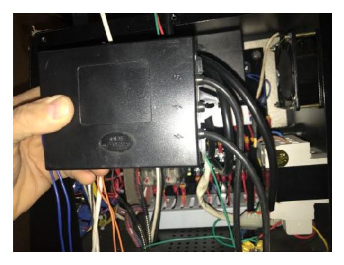
Then the next toughest part of repair is replacing the two BLACK ignitor needle wires. If you can reach and replace the two black ignitor needle wires without having to remove the firewall between drum motor and burners this will save much time.
