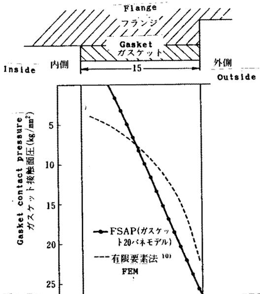
Fig. 10 Contact pressure distribution at bolt tightening phase
