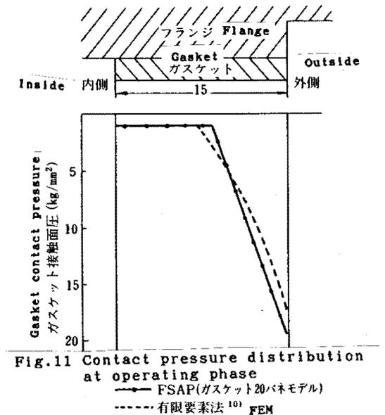
Fig. 11 Contact pressure distribution at operating phase
