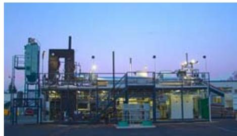
Bill Gates wants to turn your **poop** into clean drinking water, and he's got just the machine to do it. The "**Omniprocessor**", designed and built by the Washington-based engineering firm **Janicki Bioenergy**, is a steam-powered sewage processor that burns up solid waste and creates both potable water and electricity.
