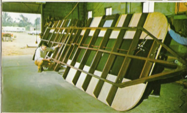
Avion has a tremendously strong triple-beam frame of heavy duty steel, including a rugged center beam for added support. Frame members are 5" deep (6" on 31 ft.).
