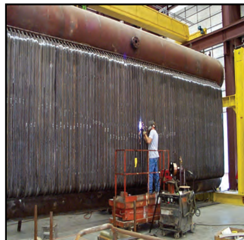
Packaged Boiler Fabrication
