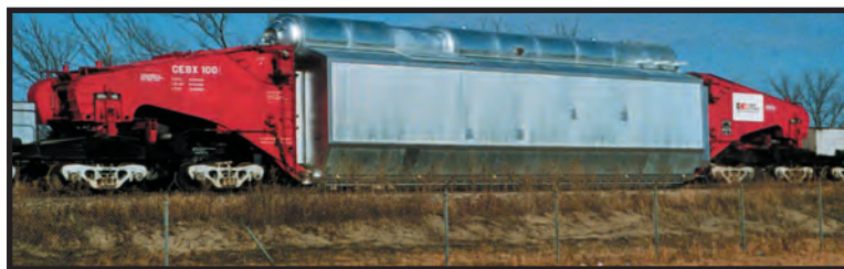
250,000 lb/hr Packaged Boiler with Schnabel Car Transportation System
