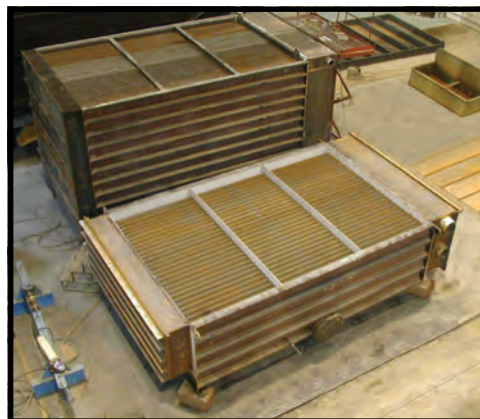
Superheater and Economizer for a Sulfuric Acid Plant
