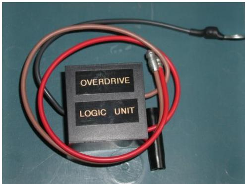
Unit fitted with Lucas connectors and also required is the double female connector so it can plug into the existing wiring under the steering column area and an earth lug to fit under a nearby nut. The unit can then be tied up under the steering column area with cable ties.
