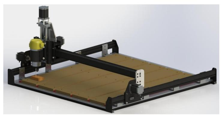
Move the block of wood out and jog it over to the front right corner. Then try and slide the block under the bit.
