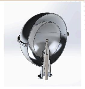
Cross-section of proposed prototype concentric AC velocity impact fusion reactor (ACVIF) with real target. To simplify, gas connections, insulation, and shields not shown.
