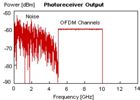
Fig. 3. RF spectrum after the photodiode. The 'noise' is due to intermodulation distortion.
