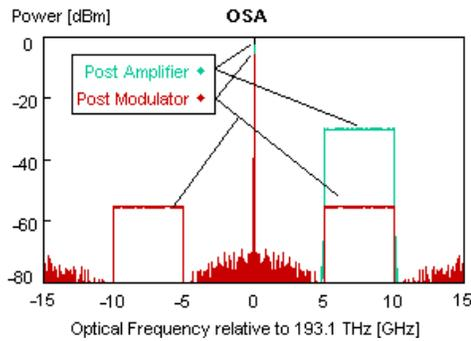
Fig. 2. Optical spectra: after modulator (dark red); after first amplifier (light green).
