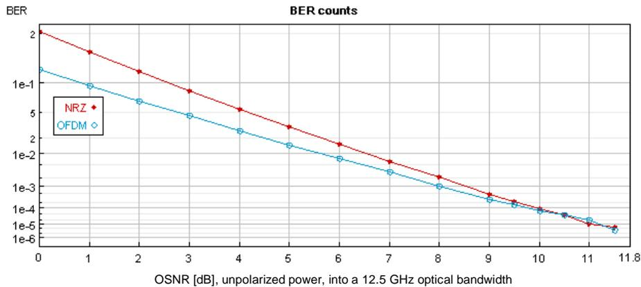
Fig. 6. BER vs. OSNR (dB) for OFDM (lower, open circles) and NRZ systems (upper, dots).
