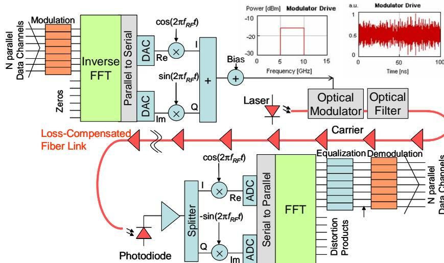
Fig. 1. Optical OFDM system block diagram.
