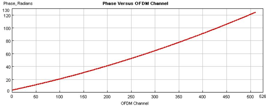
Fig. 4. Phase dependence of the fiber link stored in the training file and used for equalization.
