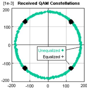
Fig. 5. Electrical constellations before and after equalization.
