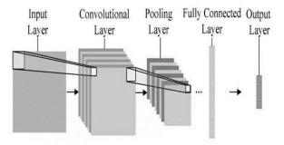
Figure.1. Basic structure of convolutional neural network.
