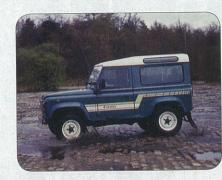
Ninety (90) completes the all-new coil sprung range. Wind-up windows are now standard and the old 2.3 petrol engine gives way to a 2.5-litre unit.
