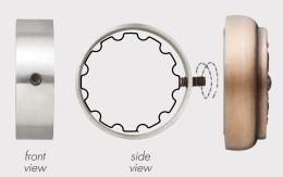
Metal band slides onto pole and is locked in place with set screw. Set screw should be positioned in the front center of pole because it receives the rosette.
