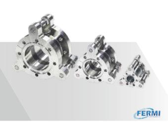
These Port Aligners enable the distance and angular relationship between two flanges to be adjusted. They are offered with three different but widely used CF standard flanges. Each type provides ±5 mm axial length adjustment, with ±3° angular tilt motion.
