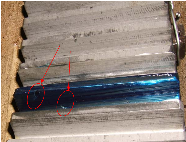
Figure 11. Ring Gear Tooth After Removing Brg Fragment & Dressing Raised Metal.
