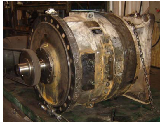
Figure 1. Gearbox On Test Stand For No Load Spin Test.
