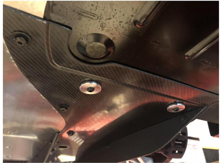
**Diffuser Hard Mount Installed (Shown Not Anodized)**
