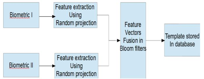
Fig.7.2: Random projection based multi biometric template protection
