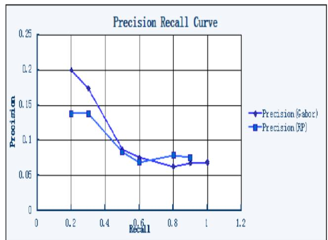
Fig.8.3: Precision recall curve for 1) Gabor filter based iris recognition system and 2) Random projection based iris recognition system.
