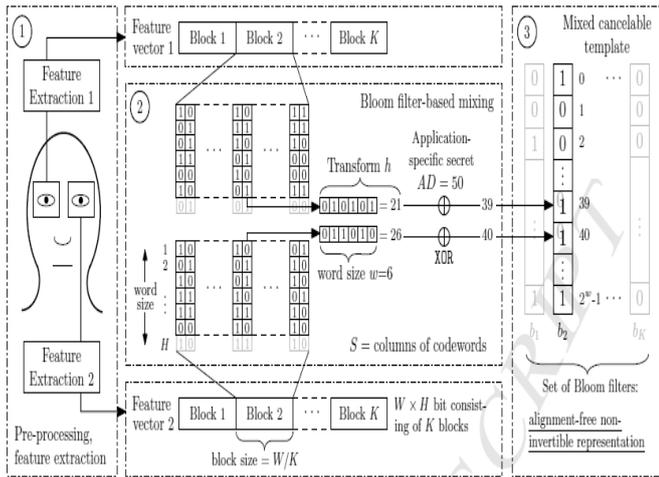
Fig.6.3: Operation of the Bloom filter based transform which mixes feature vectors of two different biometric instances [2]
