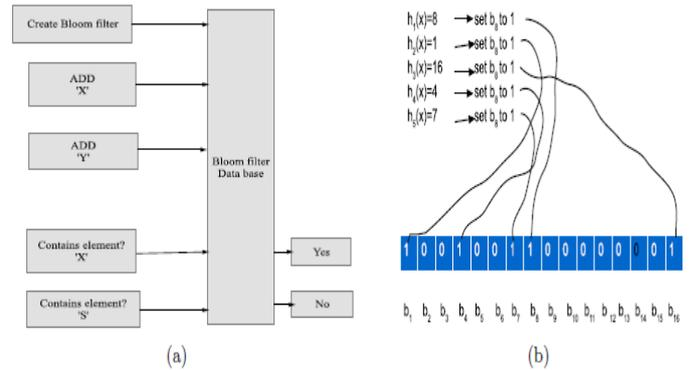
Fig.6.2: Basic bloom filter functionality
