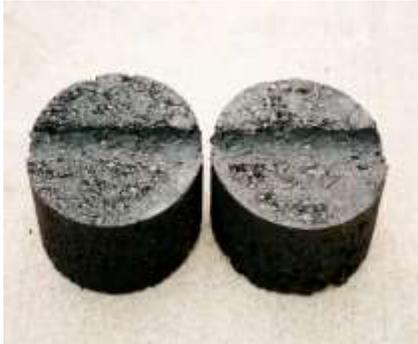
Rutted Superpave Asphalt Samples
