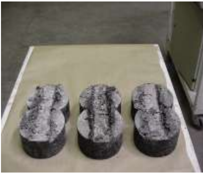
Rutted Superpave Asphalt Samples Utilizing the Hamburg Test Method AASHTO T324-14)
