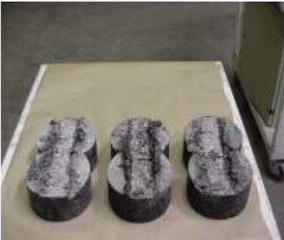
Rutted Superpave Asphalt Samples
