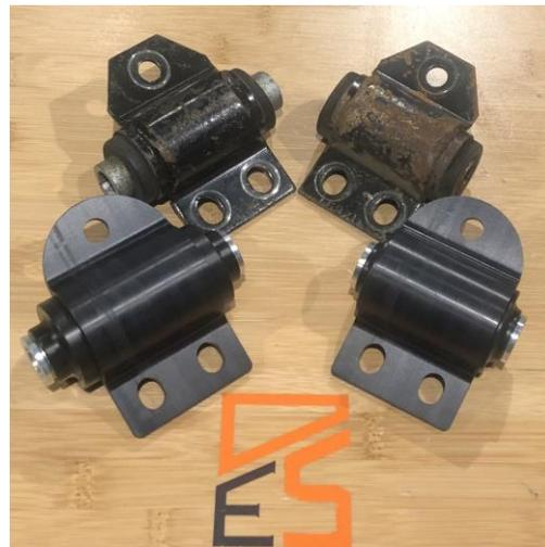
***Rear Lower Shock Mount Delrin Bushing Assembly***
